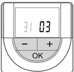
Use buttons - or + to change the value, press the OK button to set the value and move to the next editable value.
